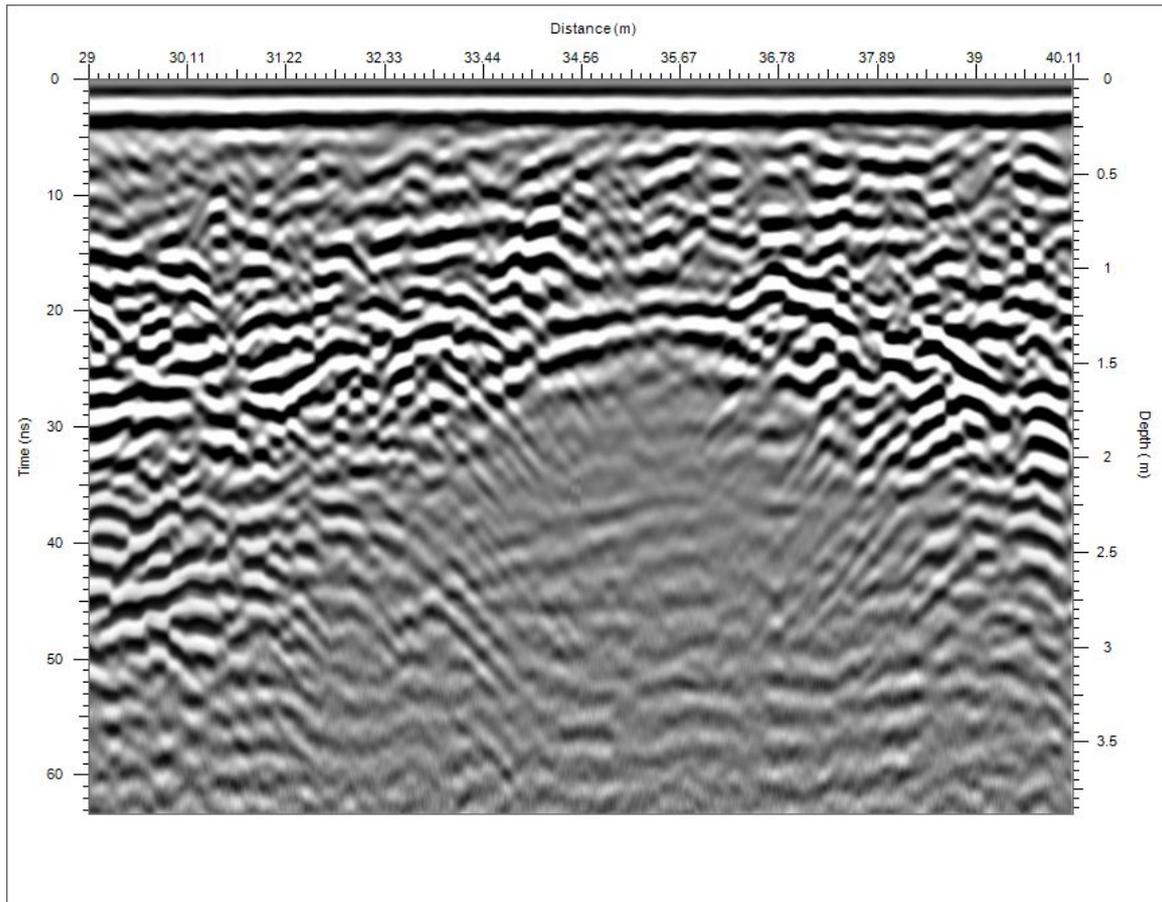
Fig. 8 The arch bridge data, it is not difficult to see where the arch is.
