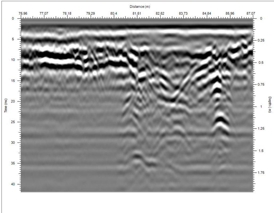
Fig. 9 The small bridge without re-bars.
